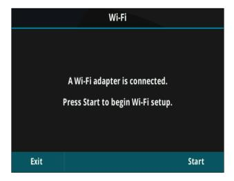
Once the device has started the above prompt will be displayed on screen, press "Start" to begin the setup.
